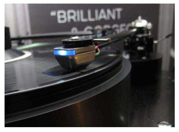
Japan-based DS Audio introduced at CES 2017 its latest optical cartridge design, the DS002 at an attractive \$5000 price point. The DS002 places the optical sensor in front of the elastomer suspension, which should produce faster response analogous to Audio-Technica's ART1000 cartridge that puts the coils on top of the stylus (not that there's really an comparison to be made between a coil and magnet based generator and one that uses an LED and optical shutter to generate a voltage).
