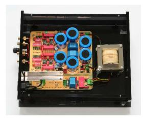
The **Mini Basis Version 2008** has be completely renewed. On the new **gold-plated** board now the AC Voltage Filter, the capacitors and amplifier part are together.
